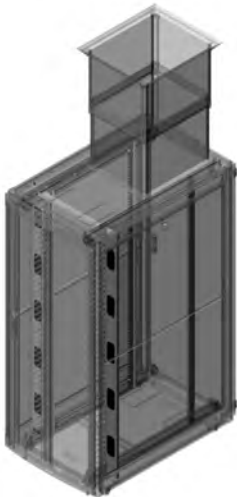
Front-To-Top Airflow - Example P/N: NX7X-XX5X-X5X-X Combine Front Air Dams with Solid Metal Rear Door and Vertical Exhaust Duct Top Panel to remove hot air through the top of the cabinet.
